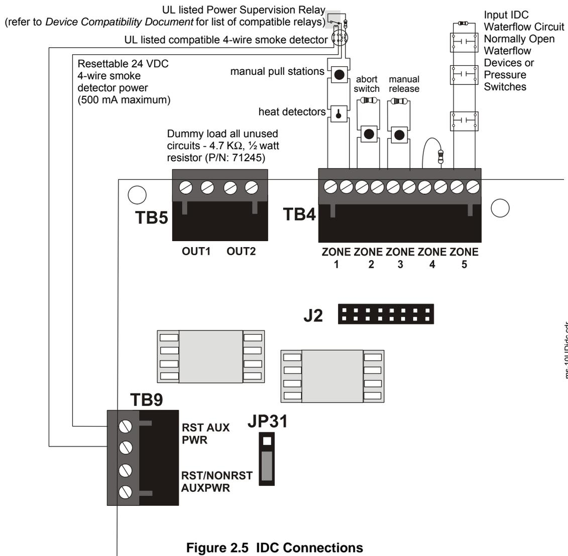
Figure 2.5 IDC Connections
