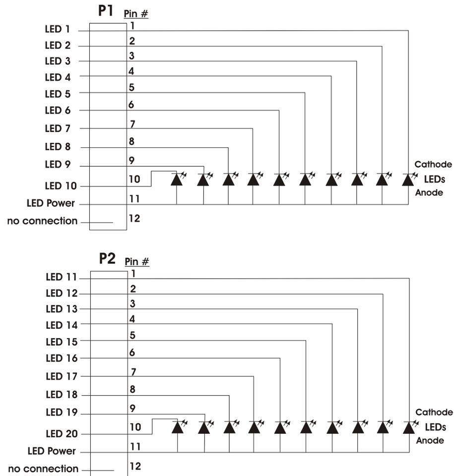
Figure 2.24 N-ANN-I/O LED Wiring
