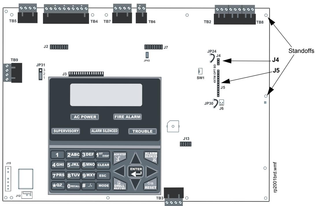
Figure 2.15 4XTM Option Module Connection
