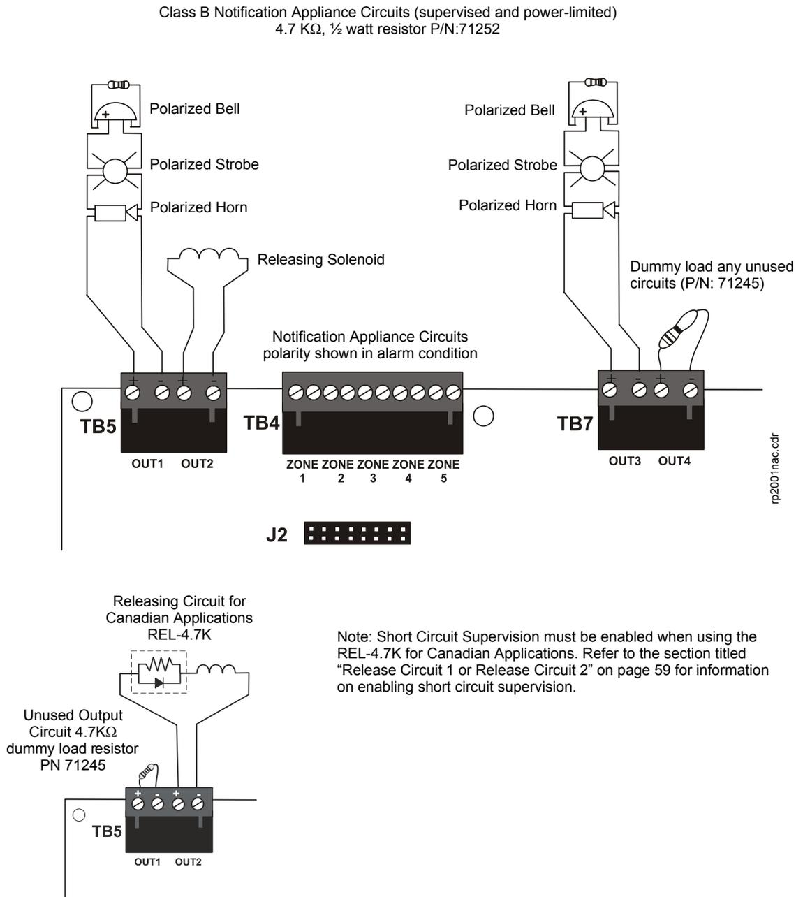
**Figure 2.8 NAC/Output Connections**
