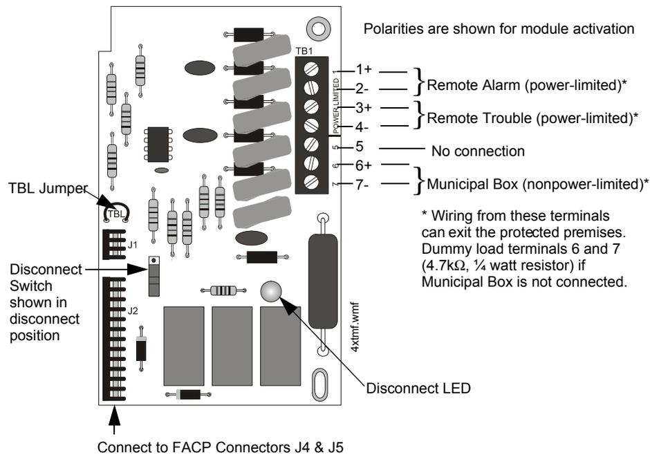
Figure 2.16 4XTM Transmitter Module
