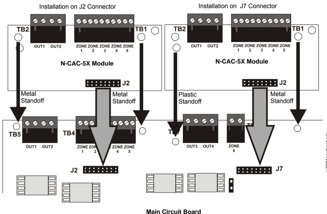
Figure 2.13 N-CAC-5X Module Installation
